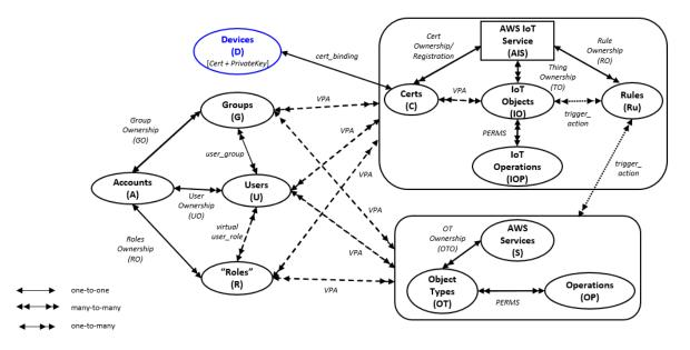
FIGURE 2. AWS-IoT access control (AWS-IoTAC) model within a single project [11].
